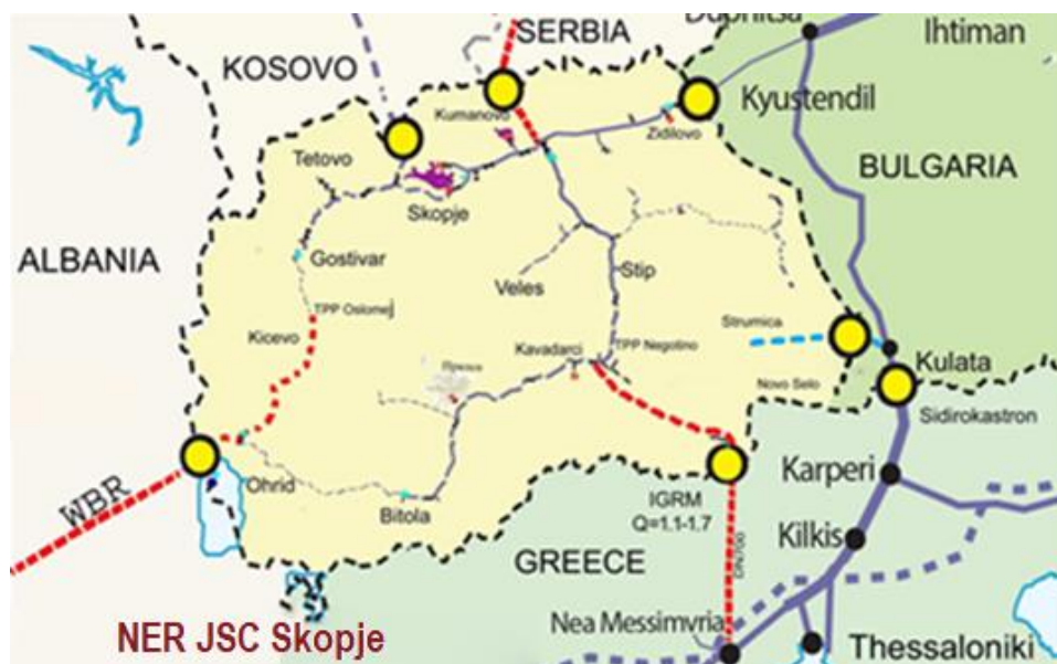
Figure 3: Routing of the pipeline from Nea Messimvria to the border with North Macedonia
